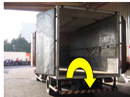
Figure 5 Example of an underrun protection bar on a transport vehicle.
